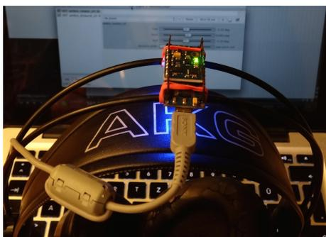
(a) Do-it-yourself drift-compensated headtracker composed of an Arduino Nano and 3-axis-accelerometer, gyro and magnetometer sensorboard.
