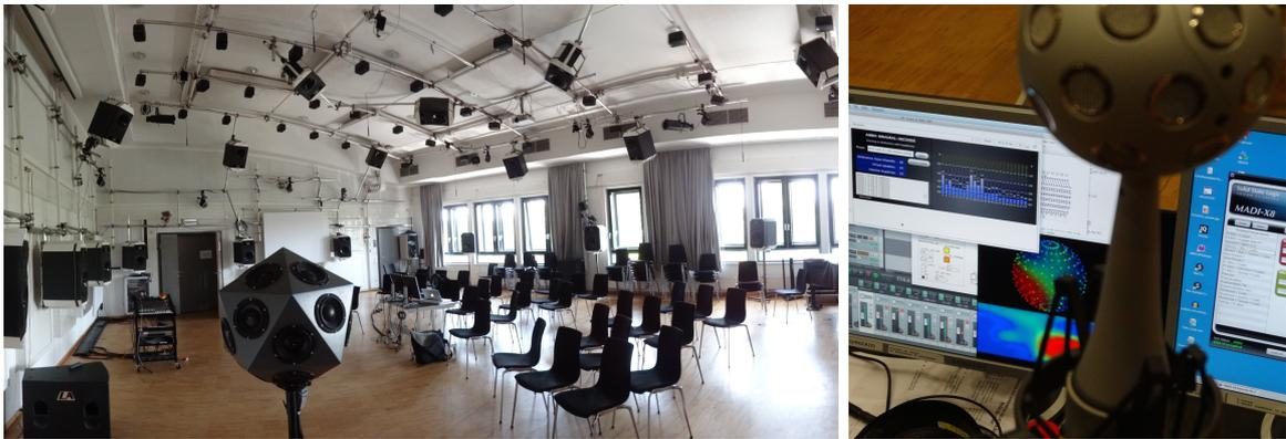
**Figure 1.1:** Hemispherical loudspeaker arrangement in the IEM-CUBE, Icosahedral loudspeaker array and mh acoustics Eigenmike<sup>®</sup> represent the motivation for this thesis.
