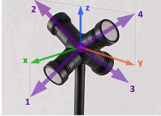
**Figure 7:** Capsule vectors representing the look direction of each microphone capsule in the local coordinate system. The picture is taken from [Okt], the coordinate system is included for clarification.
