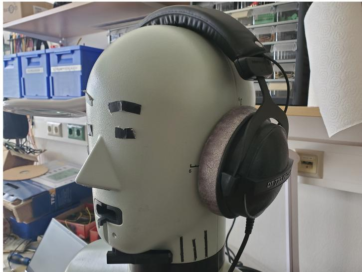
Figure 4.6: Calibration setup using artificial head
