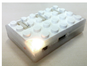
Figure 7.3.: The BRIX 2 physical computing and sensor platform. Photo: Sebastian Zehe, 2014. 5
