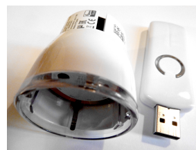
Figure 7.2.: Wall plug and wireless USB dongle for real-time electric power measurement.
