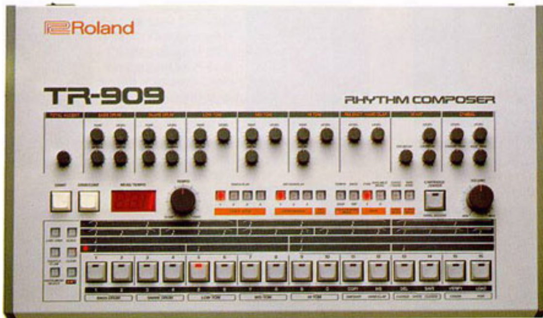
Illustration 18: Roland TR-909 ; Rhythmsynthesizer with standard step-sequencer By Eriq at Dutch Wikipedia, CC BY-SA 3.0, https://commons.wikimedia.org/w/index.php?curid=3218655
