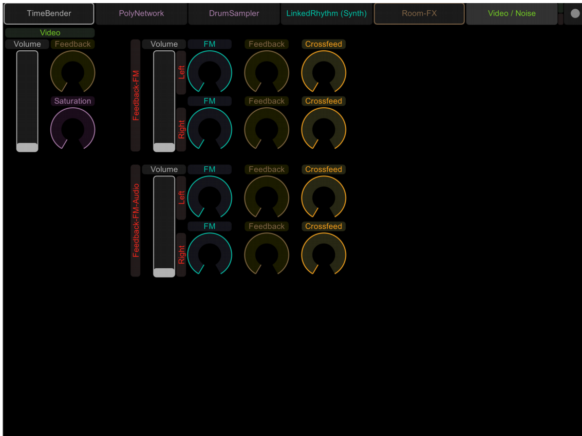
Illustration 30: Feedback-FM-Synthesis (internally, using the waveforms generated by the 'TimeBender', and externally, based on input material received from the analog-mixer)
