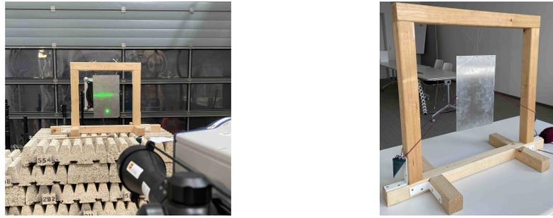
**Figure 57** – Laser vibrometer measurements (left) and built plate suspension device with aluminium replica plate  $a_1$ (right).
