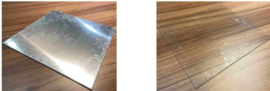
**Figure 54** – Aluminium replica plate  $a_3$  (left) and glass replica plate  $v_1$  (right).
