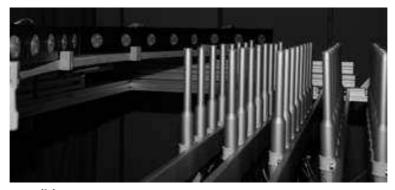
**(b)** Loudspeaker array with measurement microphones.
