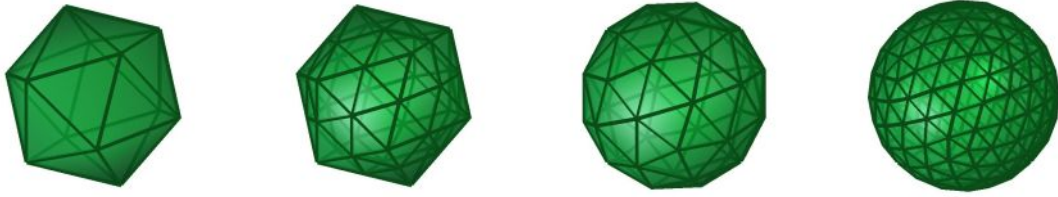
Figure 27: Building a geodesic sphere from an icosahedron
