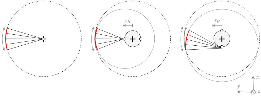
Figure 3: Isophasic monopoles driven by a degenerated beam lead to destructive interference in case of eccentric receivers, cf. [7].
