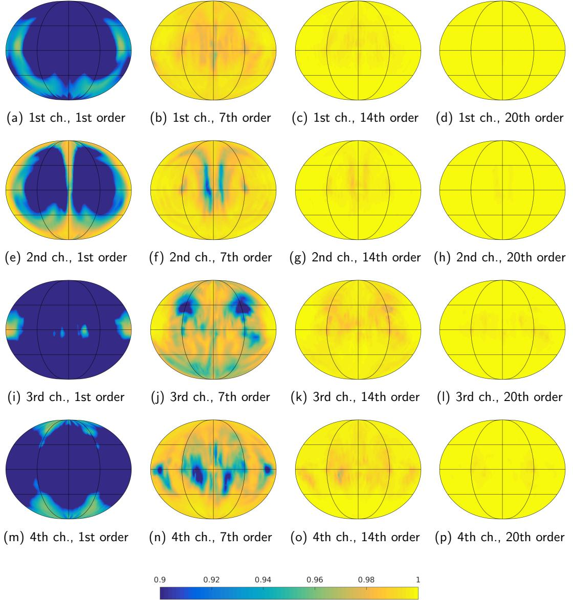
Figure 6: Correlation (angle)  $\rho_w$  between original and SH-evaluated impulse responses (minimum of left and right channel). Values below 0.9 are mapped to 0.9.
