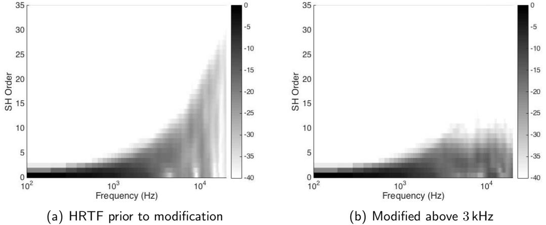
Figure 4: Relative modal energy distribution of an HRTF set over frequency and impact of ITD equalization (HRTF of Neuman KU-100, cf. [11]).
