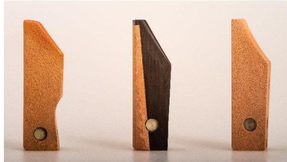
Photo 90: three blocks in comparison standard Synpor, Combi block, curved Synpor
