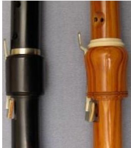
Photo 11: straight and bent key for the bottom note by the Kehr workshop
