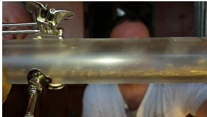
Photo 64: acrylic glass Helder Tenor used for Kundt's experiment
