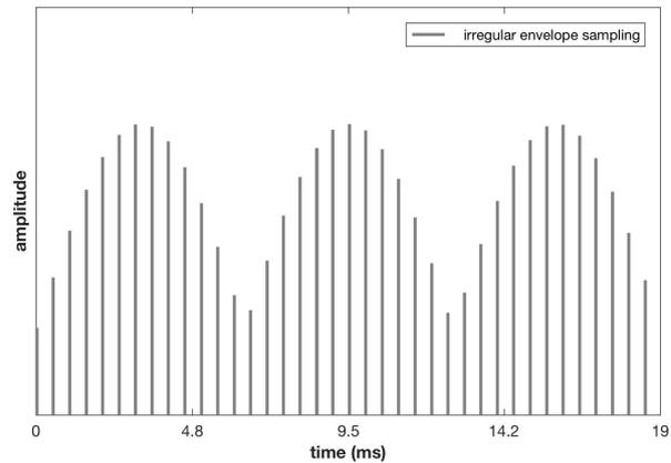
Figure 2.2 – Irregular envelope sampling: if  $i = \frac{T_{AM}}{T_c} = \frac{f_c}{f_{AM}} \notin \mathbb{N}$ .
