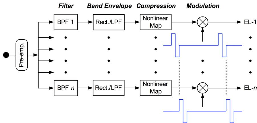
Figure 1.1 – Signal processing in current CIs (Wilson and Dorman 2008).
