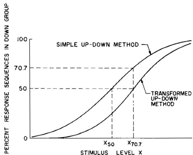
Figure 2.8 – Response curves for a simple up-down and a transformed 2-down 1-up method (Levitt 1971).
