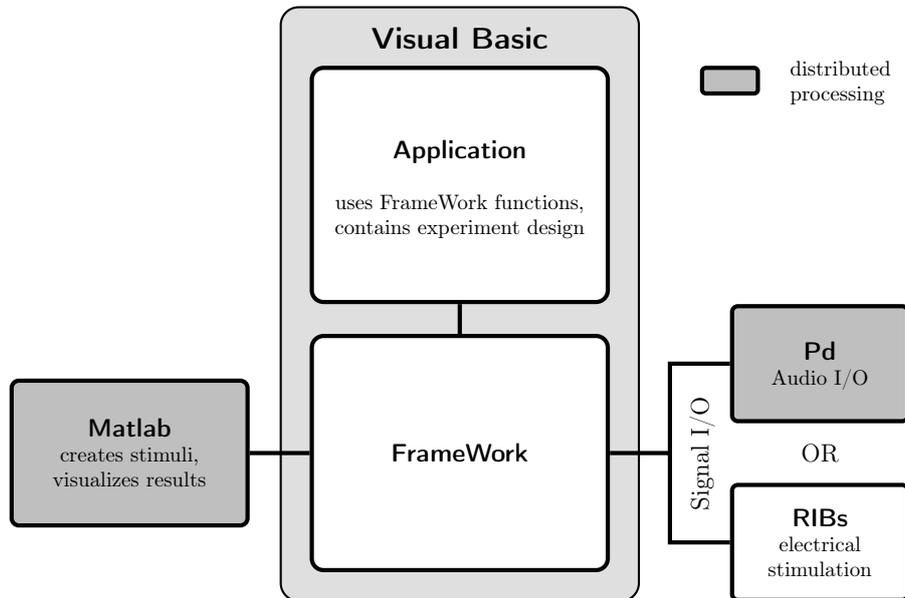
Figure 2.11 – Components of the ExpSuite software for the Pitch SIPI experiments, modified from Mihocic (2014).
