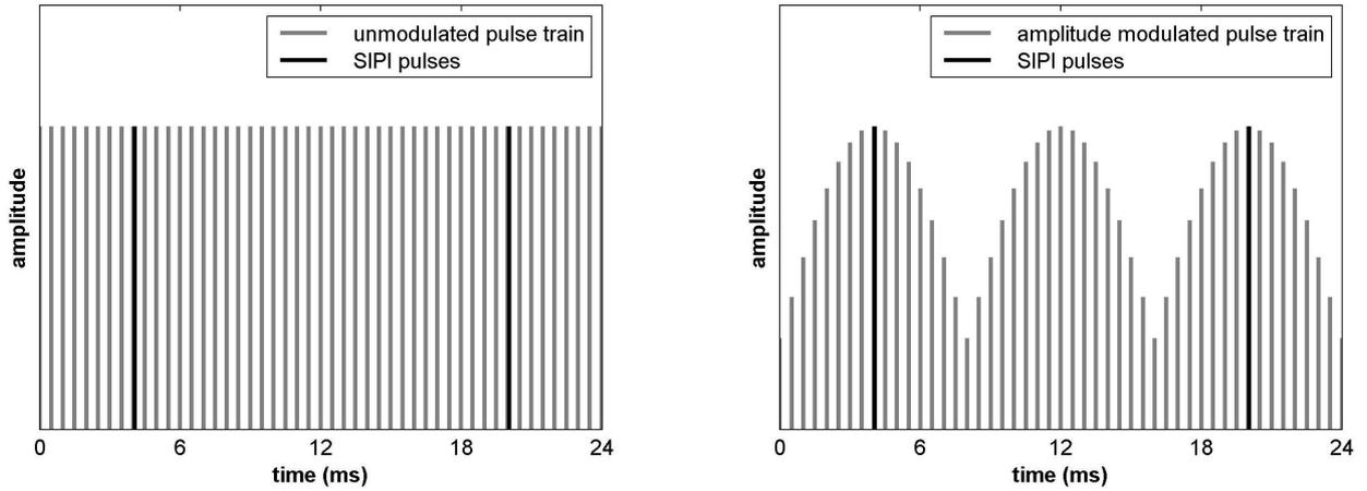
Figure 2.6 – Half Rate SIPI condition: inserted SIPI pulses with half the AM rate.
