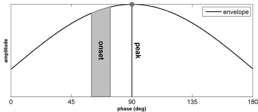
Figure 2.4 – SIPI phase conditions: peak phase ( $90^\circ$ ) and range of phases between  $60^\circ$  and  $74^\circ$  corresponding to the onset phase condition.
