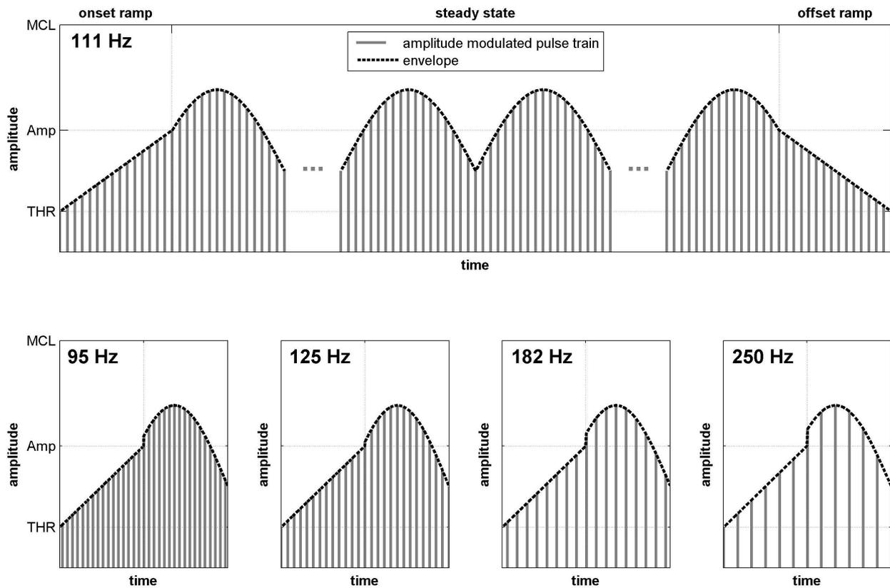
Figure 2.3 – Structure of the stimuli: onset and offset ramp, discontinuities at the beginning of the steady state part with variable length. Depending on the modulation frequency, the starting phase of the first AM period and the stopping phase of the last AM period vary as well as the length of the steady state part.
