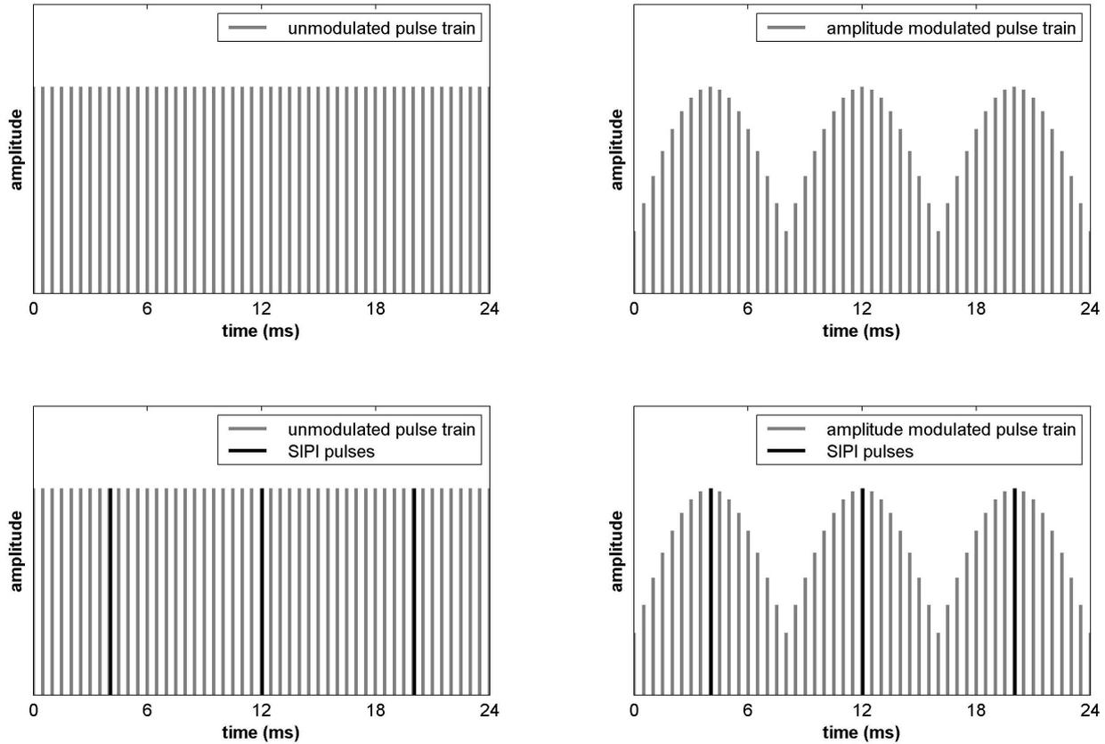
Figure 2.1 – Positive phases of electric pulse trains: *top left*: unmodulated 2-kHz pulse train; *top right*: 2-kHz pulse train, amplitude modulated with a rate of 125 Hz; *bottom left*: unmodulated 2-kHz pulse train with SIPIs inserted with a rate of 125 Hz; *bottom right*: 2-kHz pulse train, amplitude modulation and SIPIs with a rate of 125 Hz.
