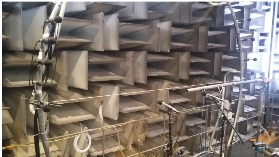
**Figure 3.2:** The acoustic measurements setup: (above) the loudspeaker box placed at the end of a side-branch pipe, (below) the semi-circular microphone array placed around the opening of the end-pipe and the two reference microphones inside the anechoic chamber.
