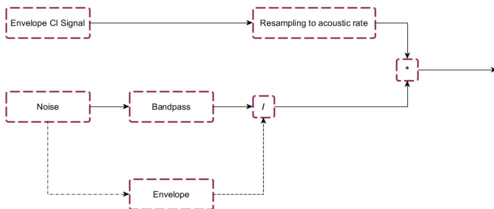
Figure 15: Sketch of the noise vocoder with removed envelope for each frequency band
