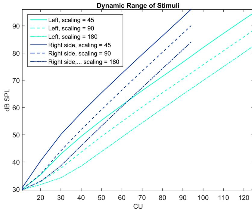
Figure 51: Acoustic output level as a function of CI stimulation level. In order to reach output levels which evoked a perception of 'very loud', the amplifier was used with a boost of 30 dB.
