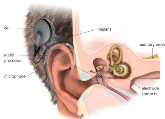
Figure 3: Schematic figure of a cochlear implant, including microphone, audio processor, coil and electrode.<sup>4</sup>
