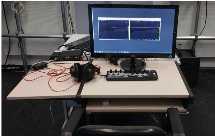
Figure 7.3: Experiment Setup: Behringer X-Touch Mini, AKG K712 Headphones, computer screen showing the interface of two Fabfilter Pro Q2 equalizer plug-ins.
