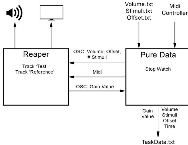
Figure 6.2: Routing and general setup in Experiment 1
