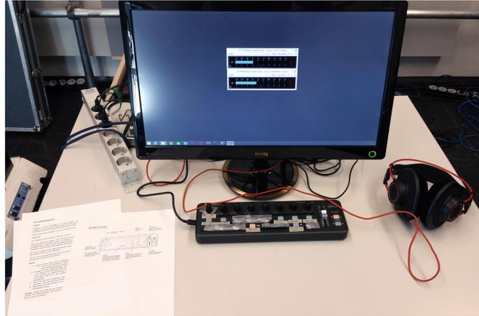
Figure 6.1: Experiment Setup; Behringer X-Touch Mini, AKG K712 Headphones, computer screen showing the interface of two PPMulator Plus loudness meter plug-ins.
