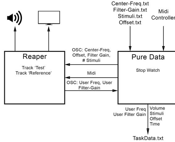
Figure 7.4: General experimental setup for Experiment 2
