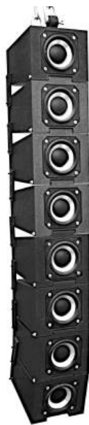
Figure 9: Fully assembled miniature line array with eight 3D printed enclosures and mounted drivers SB acoustics SB65WBAC25-4
