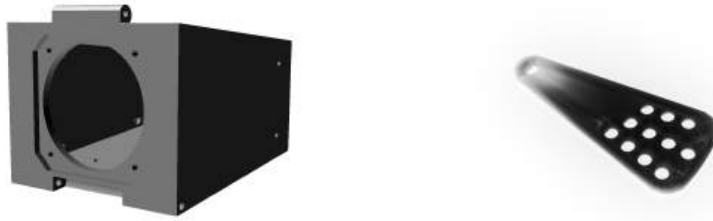
Figure 10: CAD model of a single line-array enclosure (left) and CAD model of the template for adjusting the splay angles between the line-array enclosures (right).
