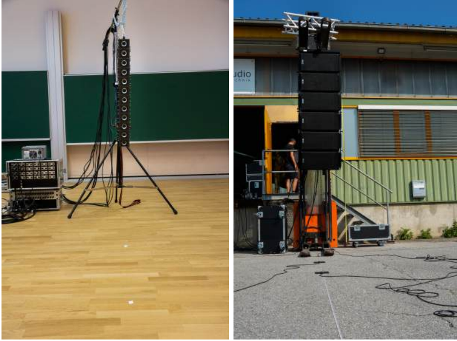
Figure 6: Measurement on the miniature line array prototype (left) and measurement on a professional Nexo Geo S12 line array (right).
