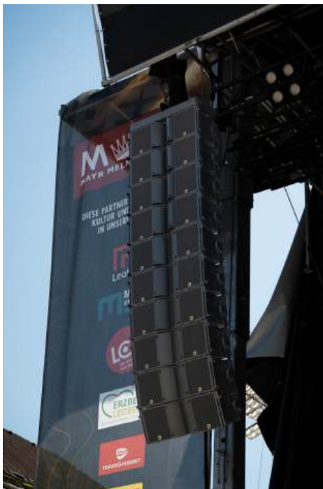
Figure 1: Example of a line-source array with ten L'Acoustics K3 enclosures, Photo: Raphael Köstl.
