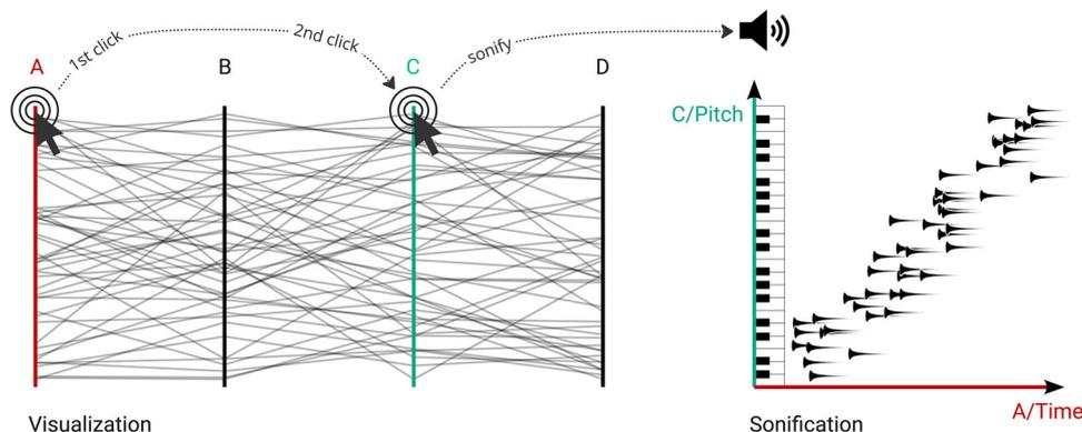
**Fig. 1** Illustration of the audio-visual analytics design *Parallel Chords* when exploring the relationship of non-adjacent axes in a parallel coordinates plot. A user selects one axis (1) which is mapped to the temporal onsets of individual sounds in the sonification, and a second axis (2)
