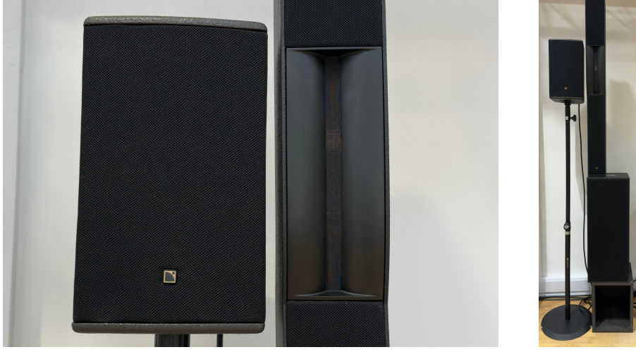
Figure 3.9: Closest possible distance (0.22 m) between HF-sections of Syva and X8, due to the pole mounting of the X8.
