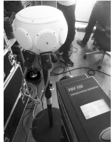
Figure 4 – Setup for the velocity measurement.
