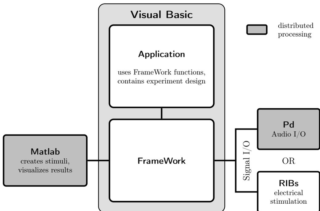
Figure 2.7 – ExpSuite software structure, modified from Mihocic (2014), taken from ?.
