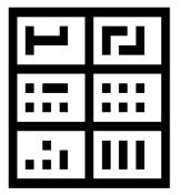
Figure 1.2 example of an fiducial marker
