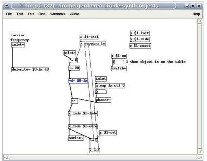
Figure 4.1 fm object implementing the phase modulation
