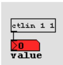
When the switch button is opened (it is not pushed down), the current at the I-cube device input is 5V and the value of the Midi controller sent to PD is 127. At the moment the button is switched, the input current changes to 0V and the controller's value changes to 0.
