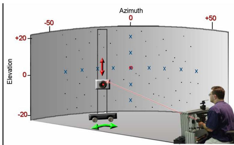
The speaker is moved randomly with a robotic arm behind the acoustically transparent screen. The listeners are asked to align the pointer with their eyes and to point to the perceived direction where the source is located. The sound location is reported with a visually-guided laser pointer.
