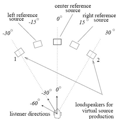
Another system to check the participants' ability in the sound localization is the method of adjustment [2]. In this experiment, three loudspeakers whose gain could be modified are set up in a horizontal plane. The gain variability causes the movement of a virtual sound sources between the arcs defined of two adjacent loudspeakers. In this case two virtual sources are created.
