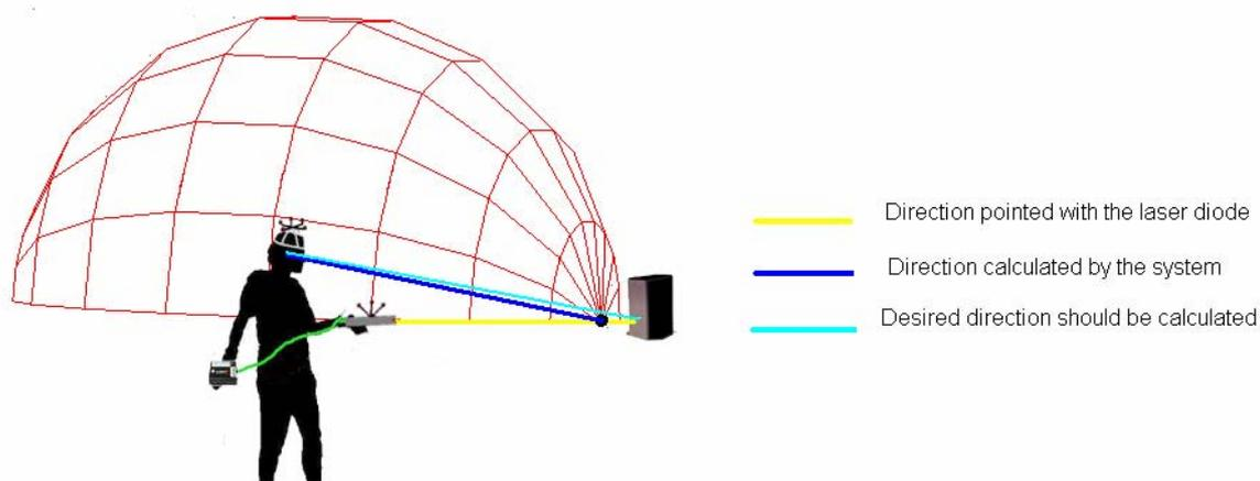
In this case the pointing device, the loudspeaker position and the intersection point are located in the same straight line.
