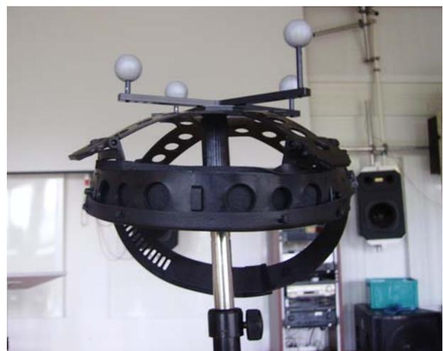
**Tracking system:** This is the tool to perform motion measurements. It provides an excellent accuracy and delivers a precise motion tracking of all objects with reflective markers.
