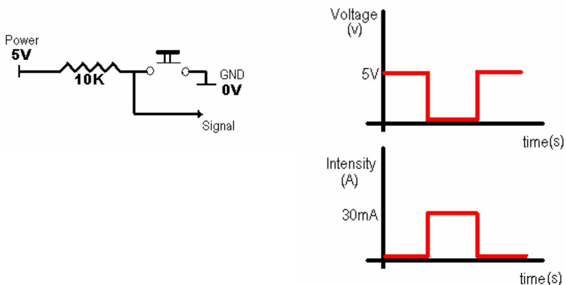
When the button is at rest the input signal is 5V and the intensity 0A. However, in the instant the button is pressed, the input signal changes to 0V and the voltage reach to a maximum of 30mA. One of the 32 inputs is used to introduce the voltage translation into the I-cube.
