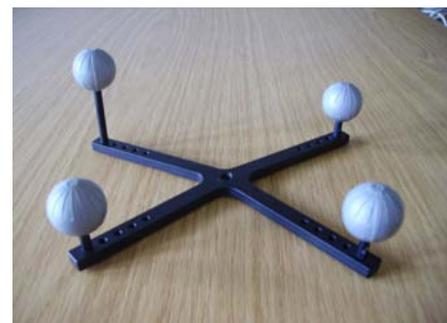
During the experiment two different capture objects are used. One is included in the pointing device. The other one is required to obtain the reference position of the listeners head.
