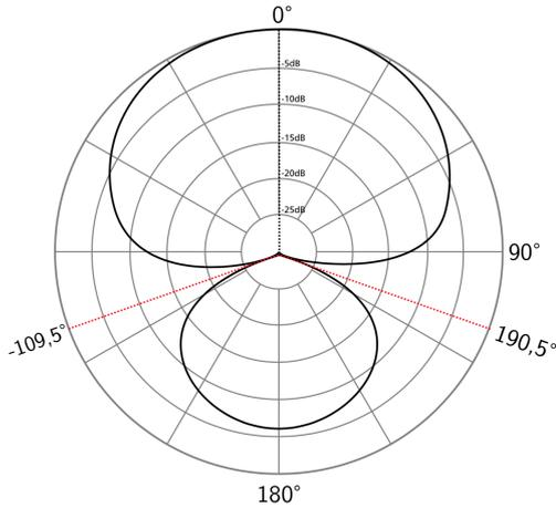
Figure 4 – 2-dim. directivity pattern of a hyper-cardioid microphone.
