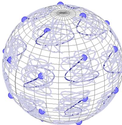
Figure 1 – Trajectories for frequency-dependent panning on a sphere, from [ZFKC14].
