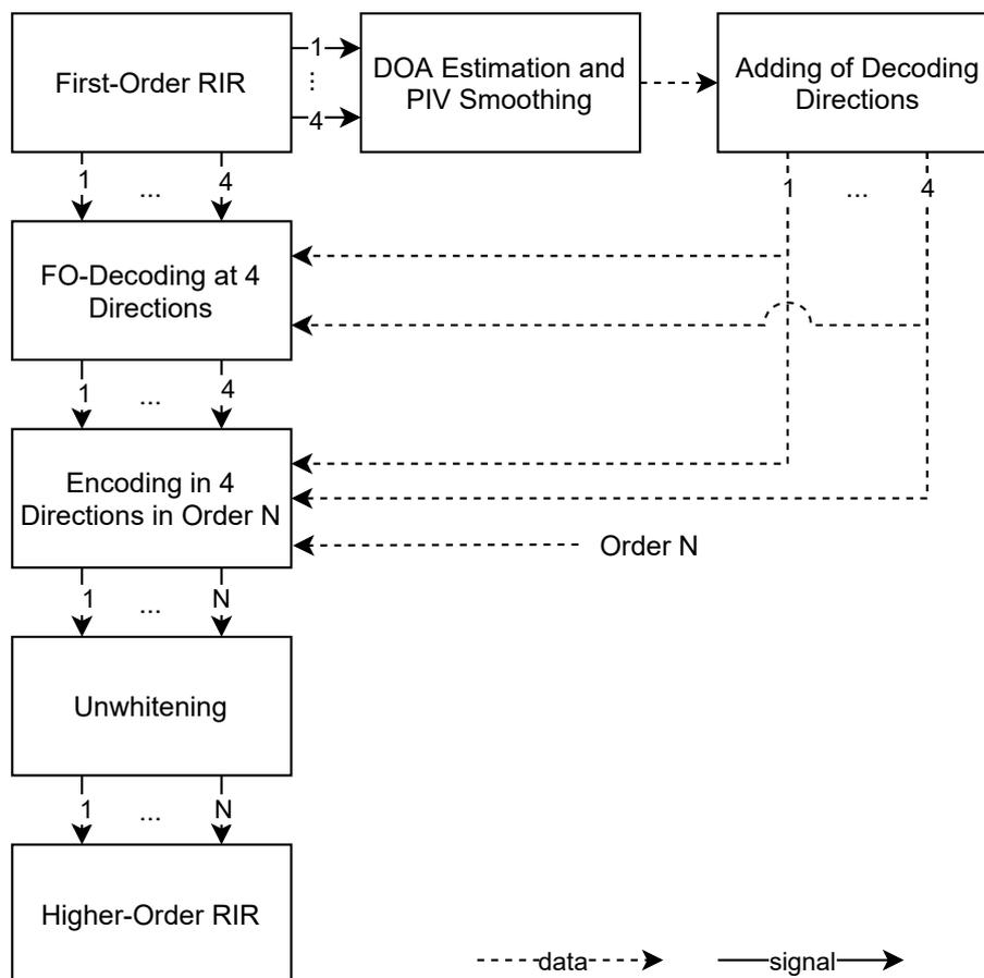
Figure 2 – Flow chart of the developed 4DE-algorithm.
