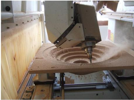
(a) milling the cone's bottom
