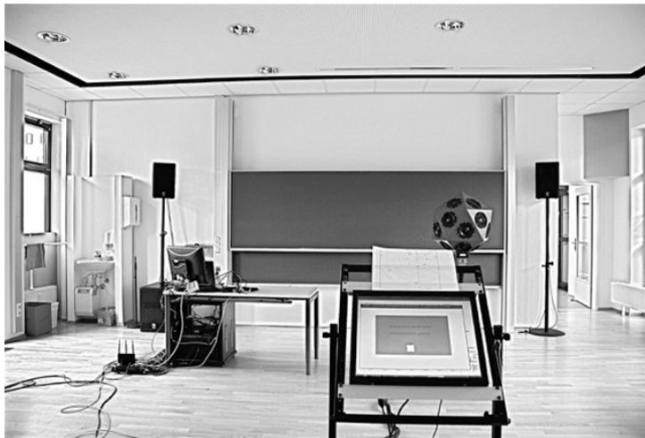
Figure 2.23: Experimental setup of Part 1 and 2 with the IKO 1 in the IEM lecture room. Answers were obtained by the marker placement on the graphical user interface shown in the foreground.
