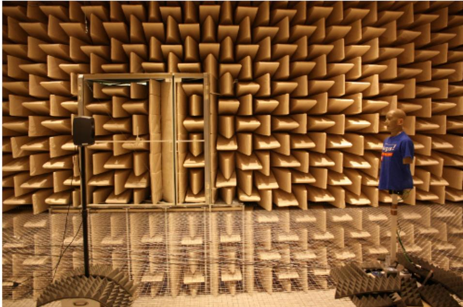
Abbildung 3: HRTF Measurement with KEMAR Dummy-Head at TU Berlin
