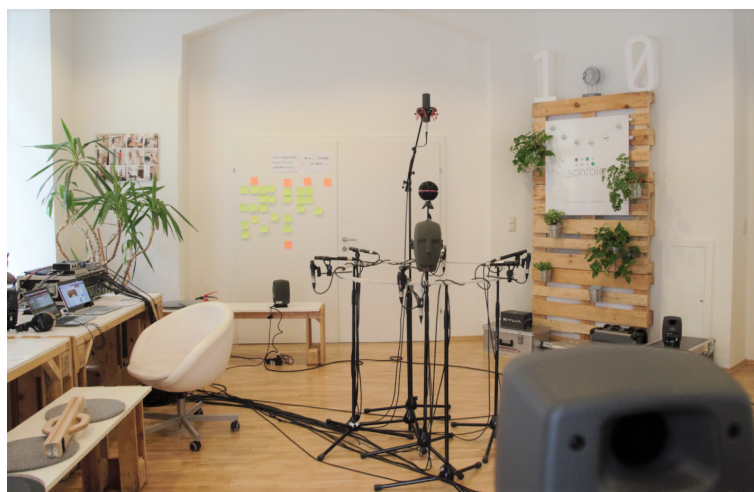
Figure 4.4 – Recording session with loudspeakers simulating an office ambience scene.
