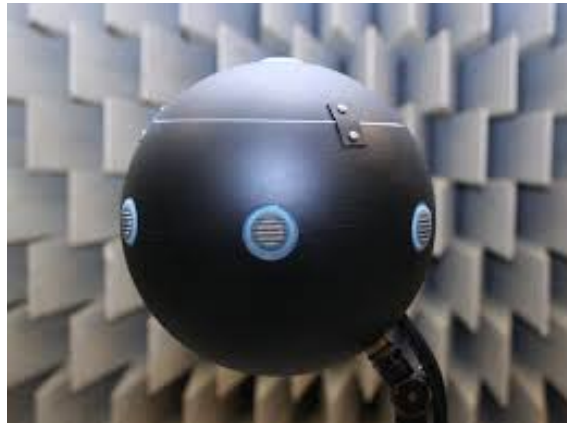
Figure 1.17 – MARVIN mixed-order microphone [MWK12].
