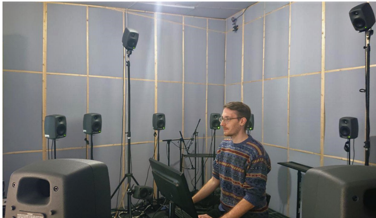
Figure 4.15 – Loudspeaker array with participant.
