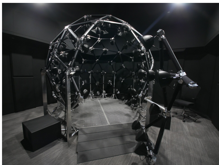
Figure 1 – 91-channel loudspeaker array in an anechoic room at the Brain and Mind Institute , University of Western Ontario designed and built by sonible
