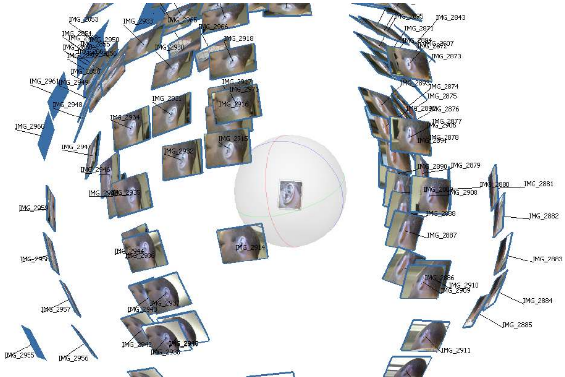
Figure 1.7: From features extracted from photos (shown as IMG_ followed by a 4-digit number), the original position of the camera is estimated. With the triangulation, a point cloud of the pinna is estimated and its shape is reconstructed. Screenshot from Metashape version 1.6.5 (Agisoft LLC).
