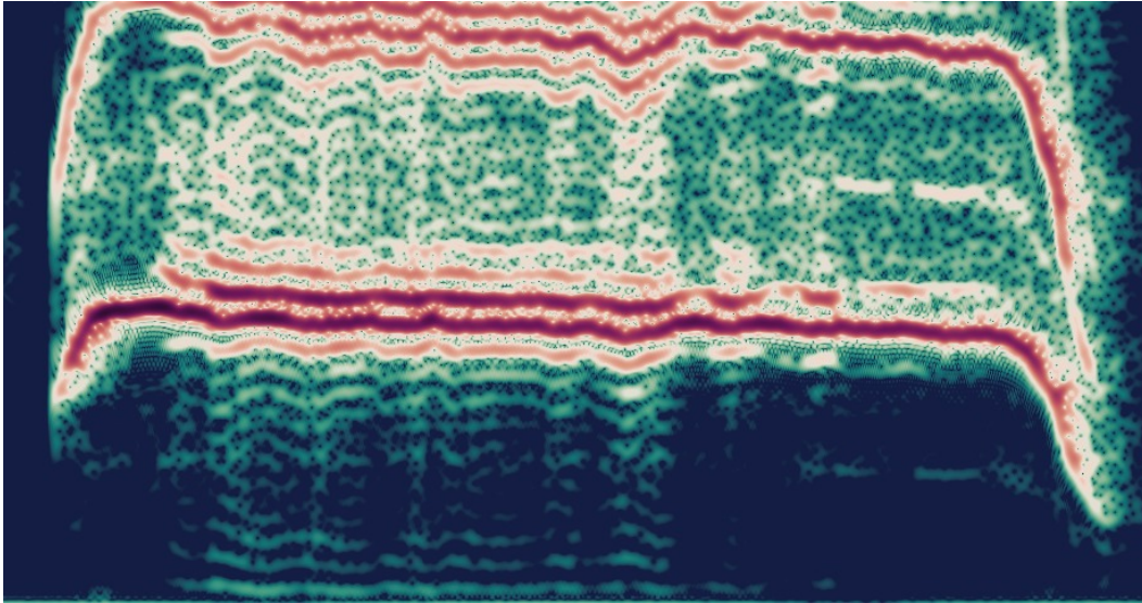
Figure 4.1: A Time-Frequency Spectrogram of a Scream, created with Python - Librosa , see chapter 5.1
