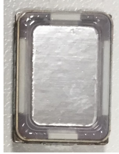
Figure 3.1 Frontal view of the 1.5 cm \times 1.1 cm \times 0.2 cm Manticore loudspeaker that was used as an alternative verification for the half-space simulations.
