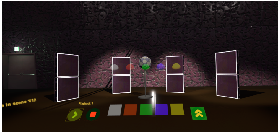
Figure 6. Screen shot of VR-rendered environment. Listener faces icosahedral loudspeaker (IKO) and uses controller to switch between conditions when moved over colored floor panels and to drag-and-drop place correspondingly colored auditory event markers (opaque/translucent for active/inactive).
