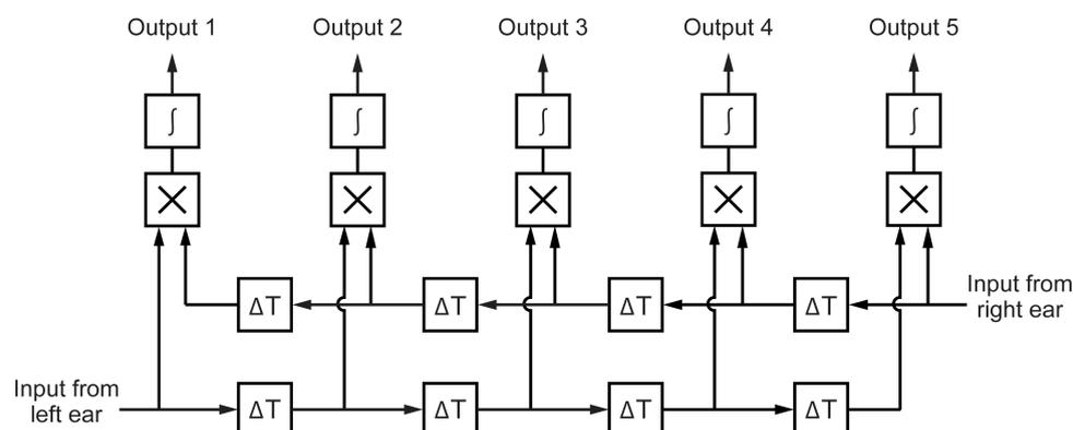
Figure 2.6: Jeffress model is presented schematically. Boxes containing crosses are correlators (multipliers) that record coincidences of neural activity from the two ears after the internal delays ( $\Delta T$ ). (Stern et al., 2005)
