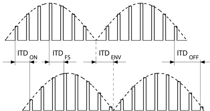
Figure 2.5: Onset ITD ( $ITD_{ON}$ ), fine-structure ITD ( $ITD_{FS}$ ), envelope ITD ( $ITD_{ENV}$ ), and offset ITD ( $ITD_{OFF}$ ) in a modulated pulsatile stimulus. Adapted from Majdak (2008)
