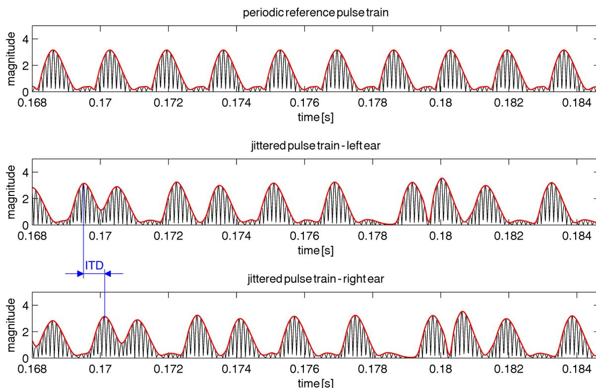
Figure 5.3: An excerpt from a 600-pps pulse train. The upper panel shows the periodic reference signal. The middle panel shows the left ear signal containing a  $k$  value of  $1/2$ , and the lower panel shows the corresponding right ear signal with an ITD of  $600 \mu\text{s}$ . The envelopes of all signals are shown in red.
