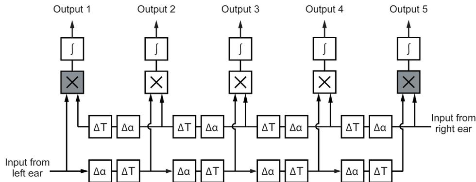
Figure 2.7: Lindemann's model is presented schematically.  $\Delta\alpha$  denotes an attenuator. All other conventions as in Fig. 2.6. At the two ends of the delay lines, the shaded boxes indicate correlators that are modified to function as monaural detectors. (Stern et al., 2005)
