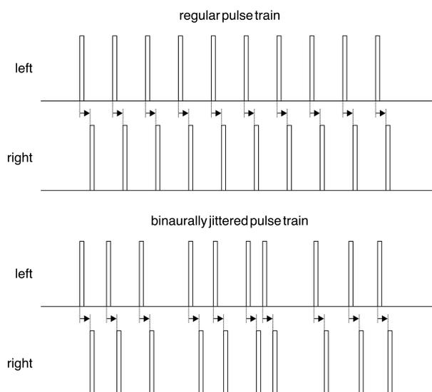
Figure 5.4: Schematics of a periodic pulse train (upper panel) and of a binaurally jittered pulse train (lower panel). Note that the binaural jitter preserves the interaural time difference. Adapted from Laback and Majdak (2008)
