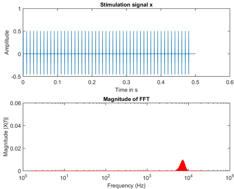
Figure 22: Stimulation signal for idealised CI listener, channel 12 with  $f_m = 7395\text{Hz}$ , the upper part shows the time signal, the lower part shows the frequency representation of the signal
