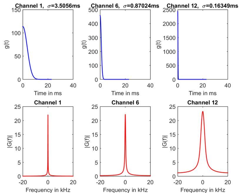
Figure 18: Gaussian pulses, upper part: time representation for three different channels, lower part: frequency representation for three different channels.
