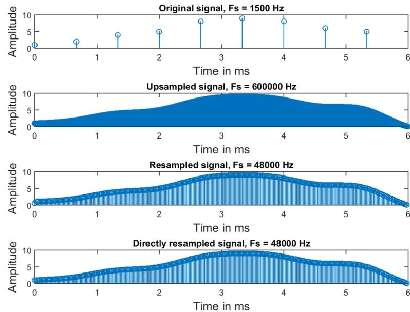
Figure 11: Re-sampling problem of electric stimuli. The first panel of the figure shows the original signal, the second panel shows the electric signal at a sampling rate of 600 kHz and the last two panels show the signal at the acoustic sampling rate of 48 kHz.
