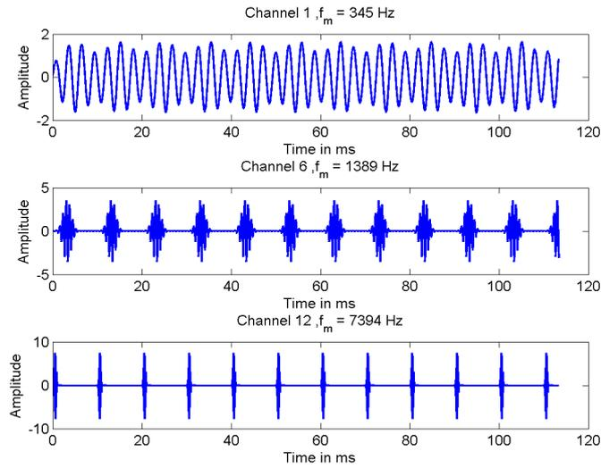
Figure 16: GET vocoder with pulse rate of 100 pps. Upper part: channel one, GET pulses were first set, summed up and then modulated, middle part: channel six, GET pulses were modulated and then set at the given pulse rate, lower part: channel twelve, same processing as channel six.
