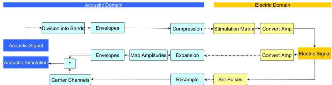
Figure 9: Sketch of converting acoustic signals into electric stimulation signals and converting them back into an acoustic simulation.
