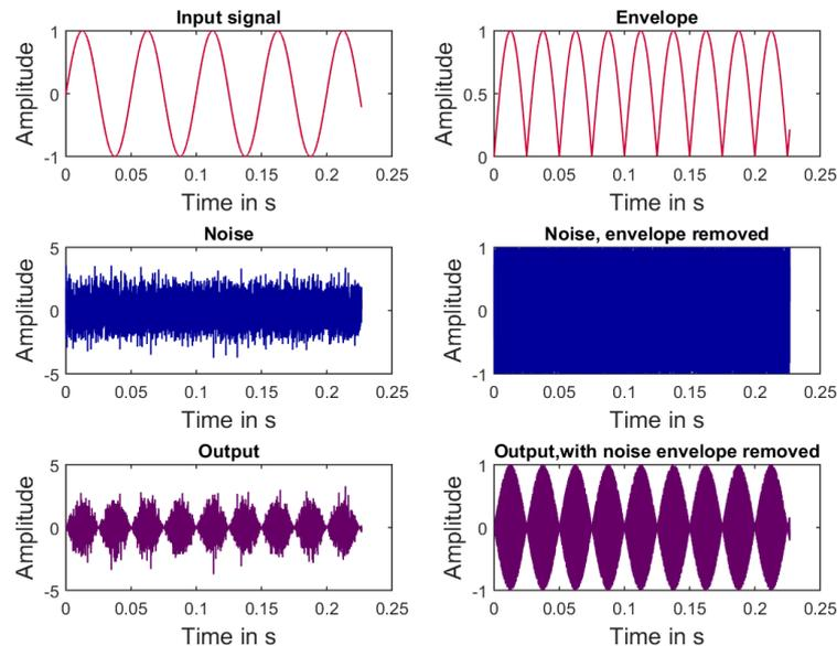
Figure 14: Effect of noise envelope removal. Upper left: input signal, upper right: envelope of the input signal, calculated using the Hilbert transform. Middle left: noise carrier, middle right: noise carrier with removed envelope. Lower left: envelope multiplied with original noise carrier, lower right: envelope multiplied with noise carrier with removed envelope.
