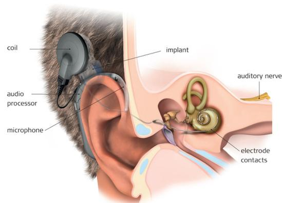
Figure 3: Schematic figure of a cochlear implant, including microphone, audio processor, coil and electrode.<sup>4</sup>
