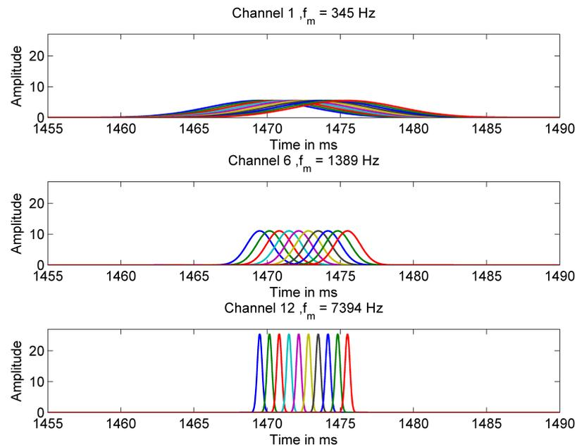
Figure 19: Failure of the GET vocoder at a pulse rate of 1500 pps for channel one, six and twelve. For all channels, the overlap of pulses is too large to keep the characteristics of the single pulses.
