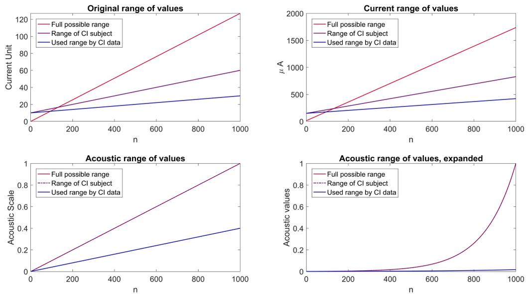
Figure 13: Conversion of levels for three different ranges: full range of 0 to 127 CU (red), full range of THR = 10 to MCL = 60 (purple), and partially used range of THR = 10 to MCL = 60 (blue). CU are shown in the top left panel, current levels are shown in the top right panel, acoustic levels are shown in the lower left panel and acoustic levels with expansion are shown in the lower right panel.
