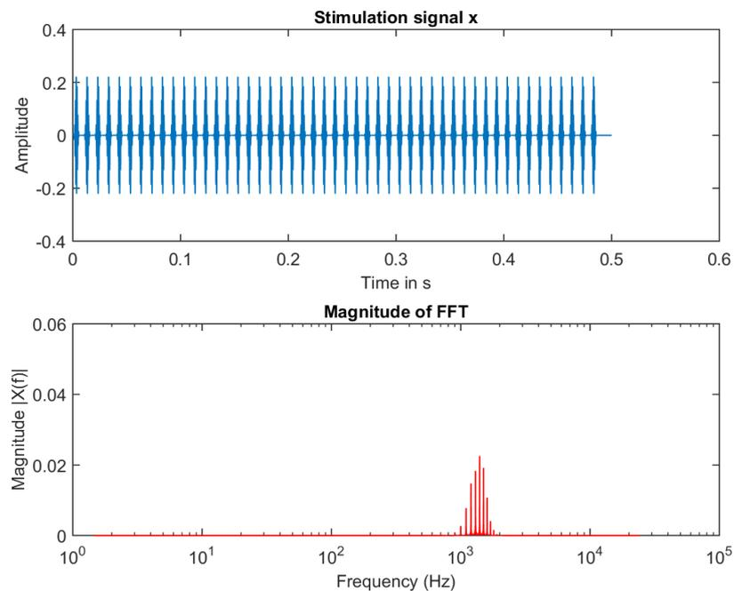
Figure 21: Stimulation signal for idealised CI listener, channel 6 with  $f_m = 1389$  Hz, the upper part shows the time signal, the lower part shows the frequency representation of the signal
