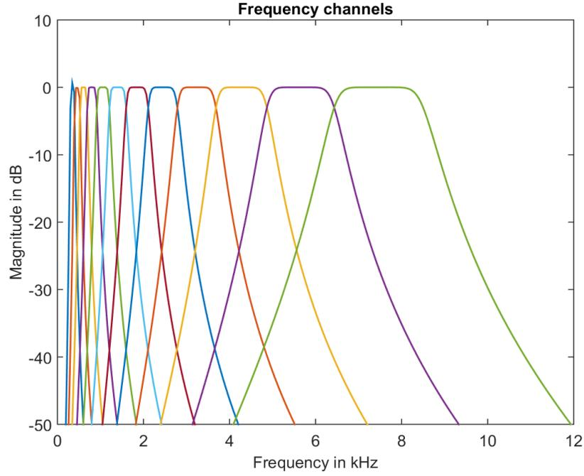
Figure 12: Filterbank with twelve fourth-order Butterworth filters, which were placed logarithmically on a frequency scale from 300 Hz to 8500 Hz.
