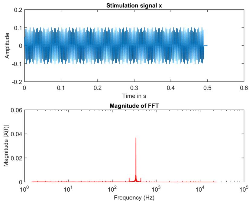
Figure 20: Stimulation signal for idealised CI listener, channel 1 with  $f_m = 345$  Hz, the upper part shows the time signal, the lower part shows the frequency representation of the signal
