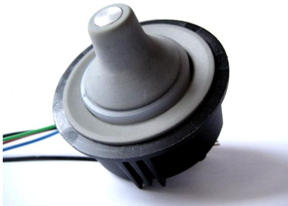
Figure 6.14: Assembled rotary encoder module
