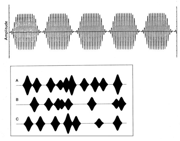
Technical Example 3.2 Quasi-synchronous granular synthesis.<sup>51</sup>
