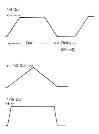
**Technical Example 3.3** Grain Envelopes with specifiable offsets between 1/4 to 1/16 the duration of the grain. <sup>56</sup>
