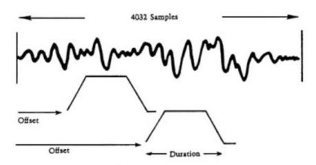
**Technical Example 3.4** Granular Time-Stretching Using a Short Fixed Sample.<sup>57</sup>
