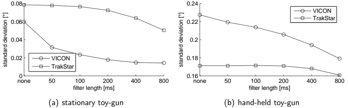
Figure 3: Standard deviation of angle error for different smoothing filter lengths.
