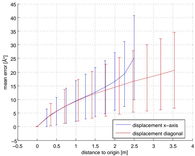
Figure 12: Deviation of the resulting direction when using the approximate model relative to the values of the triangulated vertex hull model.
