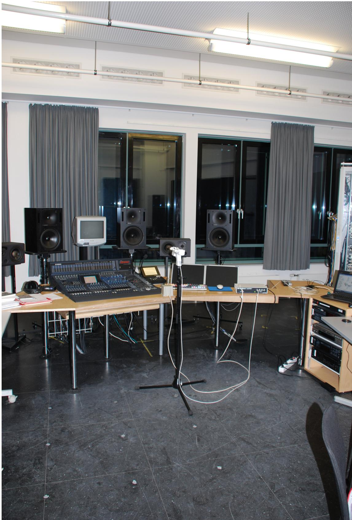
Figure 6: Measurement setup for static accuracy in the production studio, measurement positions marked on the floor.
