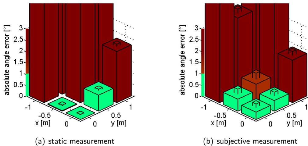
Figure 8: Absolute error of the Ascension TrakStar for both stationary and subjective tests. Depiction of standard deviation and mean as in Fig. 7.
