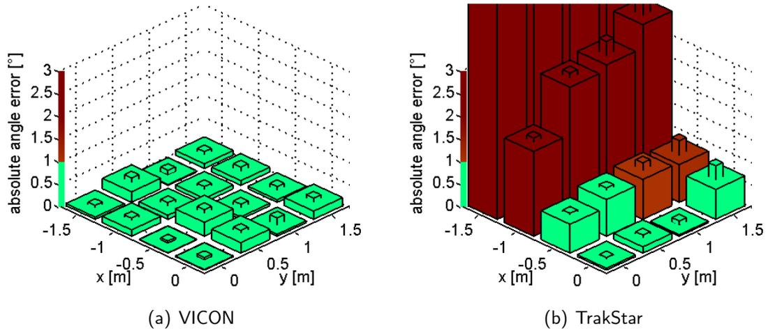
Figure 7: Absolute error for the stationary toy-gun in terms of mean (big bar) and standard deviation (small bar), sum of mean and standard deviation indicated by color.
