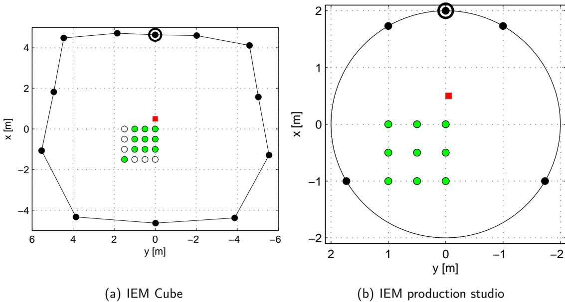
Figure 5: Measurement setups: measurement positions (green), additional positions for static tests (white), TrakStar transmitter (red square), lowest plane of vertexes/loudspeakers (black), the optical target is encircled.
