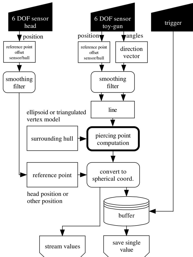
Figure 2: Complete flow chart of the calculation of the indicated direction.
