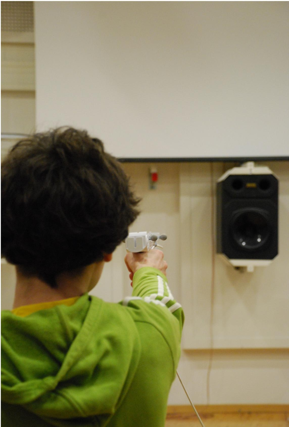
Figure 9: Aiming using the iron-sights during the subjective accuracy measurements.
