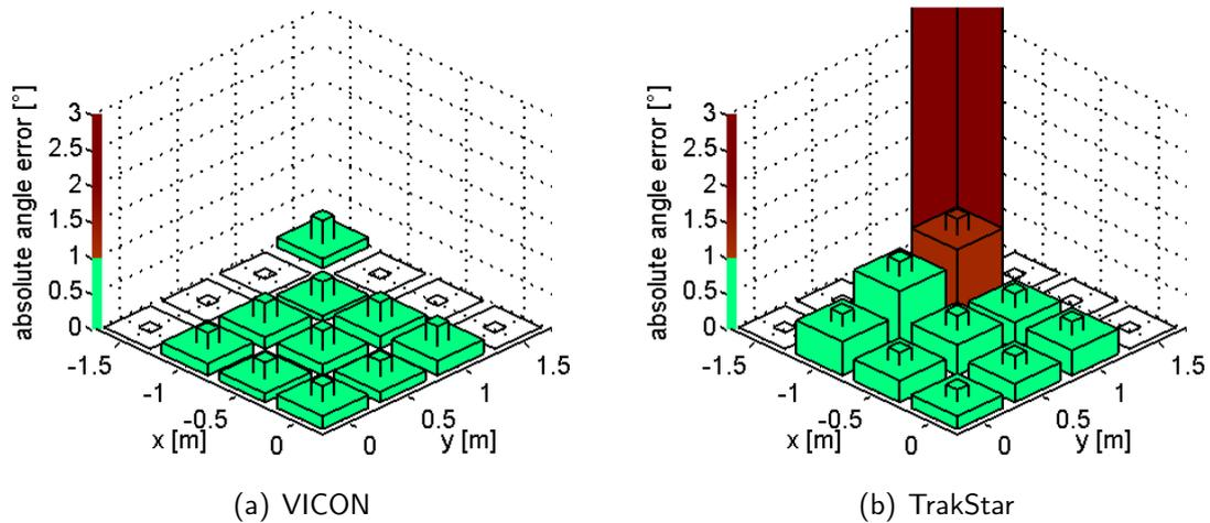
Figure 10: Absolute error for the hand-held toy-gun in terms of mean (big bar) and standard deviation (small bar), sum of mean and standard deviation indicated by color.
