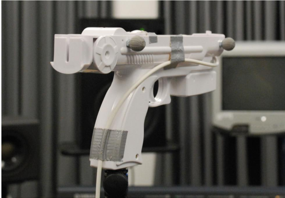
Figure 1: “WiiVolver” toy-gun equipped with retro-reflective markers and a game controller, mounted on a microphone stand.
