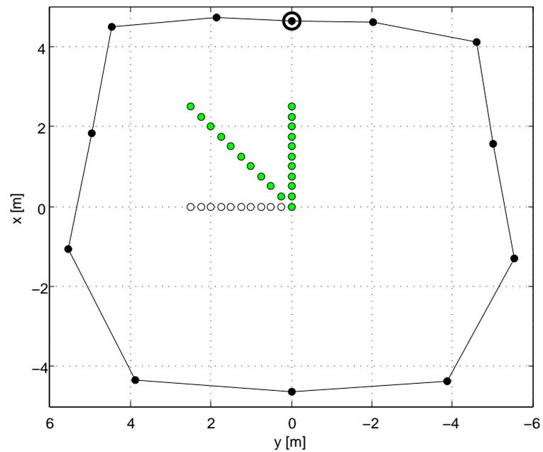
Figure 11: Measurement positions for the model comparison. Figure 12 shows the results for the points along the x-axis and along the diagonal.
