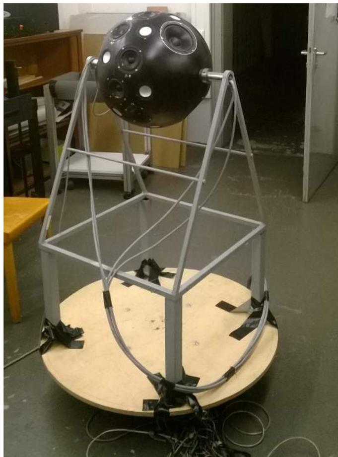
Figure 2.1: Flexible highly directive source
